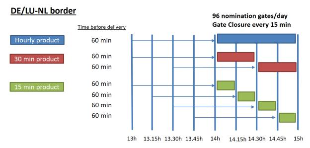
Figure 2 - Illustration of 15, 30 and 60 minutes products with 96 gates on DE/LU-NL border as of 10 December 2020
