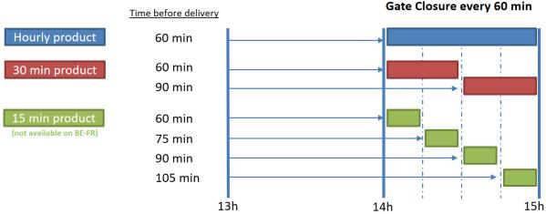
Figure 1 - Illustration of 15, 30 and 60 minutes products with 24 gates on BE-FR, BE-NL and DE/LU-BE borders as of 10
